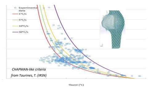
Devpt of new burst criteria (engineering or true stress based) for Zr4
