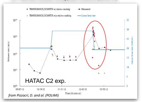
Dev<sup>t</sup> of mechanistic modelling (coupling fuel performance/FP codes for transient spike releases (due to power decrease & stress variations) (presentation 2.3 & 3.7)
