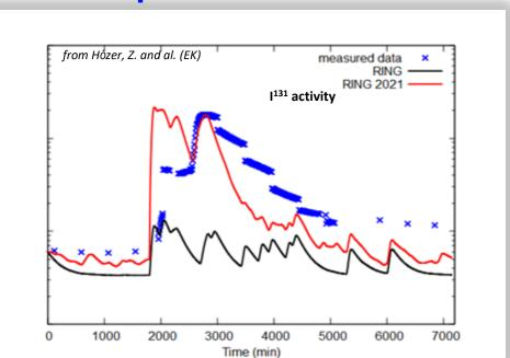
Updated correlations for lodine spike due to reactor power, primary pressure and H<sub>3</sub>BO<sub>3</sub> conc. changes from new NPP data (presentation 3.9)
