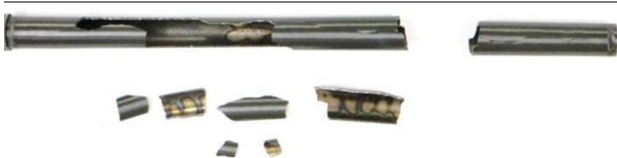
(a) Uncoated Zircaloy-4 clad segment, weight gain = 40,4 mg/cm 2
