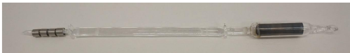
Fig. 3. The 8 mm long ring samples (on the left side) placed on the sample holder containing a soft iron core (on the right side)
