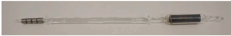
Fig. 3. The 8 mm long ring samples (on the left side) placed on the sample holder containing a soft iron core (on the right side).
